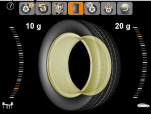
4. Manually rotate the wheel, when the inside counterweight position to green, clip the counterweight in 12 o'clock direction.
