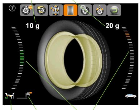
2. The indication of position of counterweight. (When the color turns from red to green, then it means we find the exact position of imbalance.)
