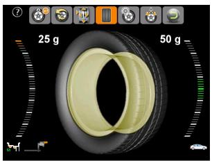
6. Follow the same process, when the outside counterweight position indicator lights turn to green, and the outside tracking sticking indicator light all on, spin the measuring scale and stick the weights on the rim.
