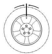
Turn the mouth of the wheel to 12 o'clock position, keep the wheel's position and confirm it by pressing OK. And the screen will show the rim's static unbalance mass, the tire's static unbalance mass, the current wheel's static unbalance mass, and the mix static unbalance mass that the wheel can reach. The user can decide to continue enhancing the wheel or not.
