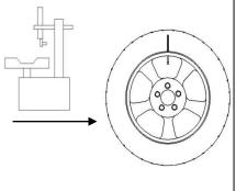
Rotate the wheel by hand, turn the balance block's position indicating piece to the top, and it turn to be red, keep the wheel's position, mark at the tire's 12 o'clock position, then take down the wheel, set it on the tire separating machine, and make the face to the air mouth of the rim.
