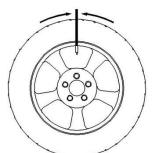
Turn the mouth of the wheel to the 12 point position, fix wheel then press [ok] for confirmation
