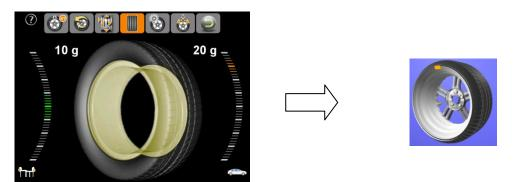
5. Manually rotate the wheel, when the outside counterweight position indicator lights turns to green, clip the counterweight in 12 o'clock direction.
