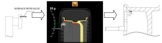
5. When doing balancing, the user must rotate the ruler to find the right position. When the right counterweight position indicator lights turn to green, and then stick the counterweight.
