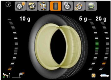
When sticking the inside counterweight, please refer to ALU-S1 counterweight pasting process. Manually rotate rim to make this two counterweight position indicator lights turn to green, and then stick counterweights to rim by measure scales.
