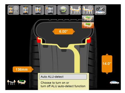
ALU automatically mode: press [ok] to activate ALU automatically mode. Under this model, the computer can identify the mode type automatically by moving scales. For customers who are get used to ALU-NORM, ALU-S1 and ALU-SA, activating this function could be more convenient. But according to different tire types, sometimes, we still need to choose ALU mode manually.
