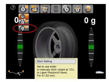
After choose laser mode, laser spot will show the place where the counterweight stick automatically when the counterweight position indicator lights turn to green. Under ALU-S1, both sides of the rim are laser position stick. Under ALU-S2, The outer side of the rim is manually stick counterweight in 12 clock direction, the inner side is laser position stick.
