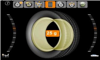
5. Manually rotate rim, when the outside counterweight position indicator lights turn to green, if it is under ALU-6 mode, then clip the counterweights in 12 o'clock direction inside of rim. If it is under ALU-7 mode, then stick counterweights in 12 o'clock direction inside of rim. If it is under ALU-8 mode, then stick counterweights in 12 o'clock direction in the middle of rim.
