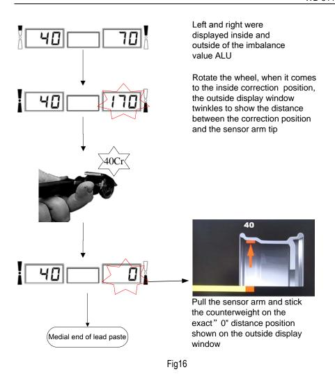
Note: The KWB-511 mechanical sensor arm can only locate the 12 o'clock position, it will return to the measurement interface if at any other position. So it is better to locate it at 12 o'clock and do the following operation.
