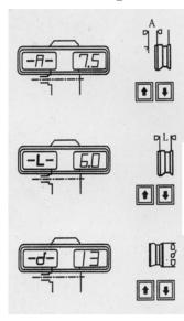
★For example testing luxurious wheel rim of Santana, please see picture on last page, use ruler that this machine has to measure distance between the machine and tyre: A=7.5cm Press ↓, number increases Press ↓, number decreases
