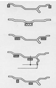
Dynamic balance: Normal- The light-alloy wheel rim of dynamic balance adopts a method of adding counterbalance at the edge of rim.
