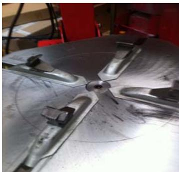
Place the tire on the clamps and press the pedal (3) to open the clamp hand thereby lock the rim. Make sure the rim is firmly fixed to the clamps.
