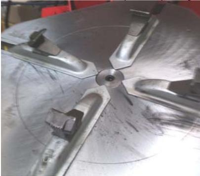
**Warning:** splitter with the clamps in the open position can be extremely dangerous for operator's hands; during the splitting operations never touch the side of the tire.
