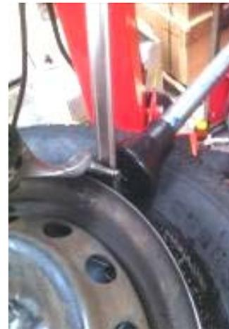
**WARNING:** In order not to damage the inner tube, if there is one, it is advisable to carry out this operation with the valve 10cm to the right of the mounting head.
