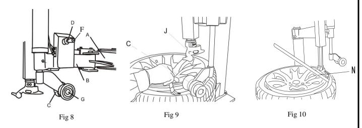
Helping arm at right side is auxiliary device of tyre changer for helping operator to demount and mount tyre.
