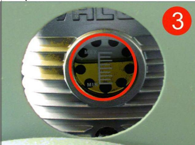
Step3: Observe the liquid level, add oil to the appropriate location
